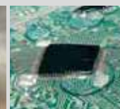
A resin-potted circuit board
